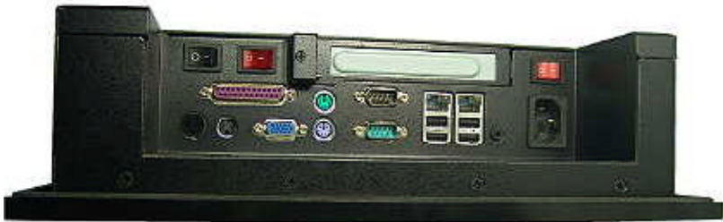
4 x USB, 4 x COM, 2 x LAN, MPEG-II, speaker, TV-out
